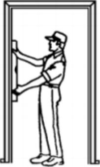
2. Checking door by opening and closing and checking hinged slot
