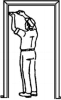
1. Pairing the door to the wall, aligned to cos, wall surface and then, open and closing M10x80
